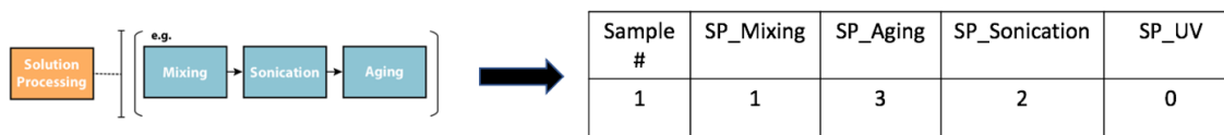
Figure 5-8. Custom approach to representing the order in which process treatments take place.
